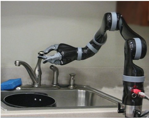
FIGURE 3-9. The KitchenBot is an overhead, track-mounted manipulator designed to aid individuals with physical impairments complete common kitchen tasks (eg, meal preparation, cleanup, etc). PHOTOGRAPH: COURTESY OF THE HUMAN ENGINEERING RESEARCH LABORATORIES, UNIVERSITY OF PITTSBURGH.
