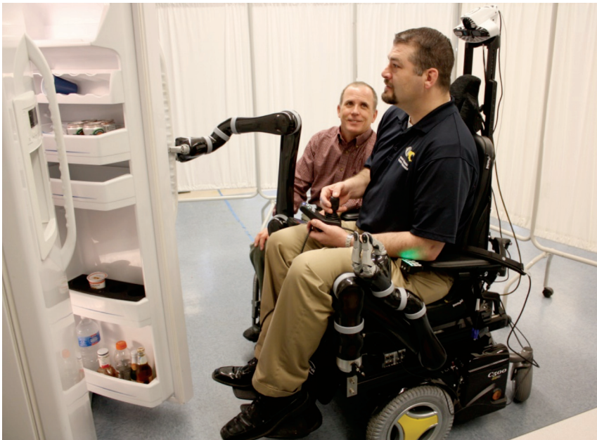
FIGURE 2-3. PerMMA is a robotic wheelchair and arm with mobile wrist and fingers. It is designed to aid those with physical impairments complete the activities of daily living. PHOTOGRAPH: COURTESY OF MICHAEL LAIN.
