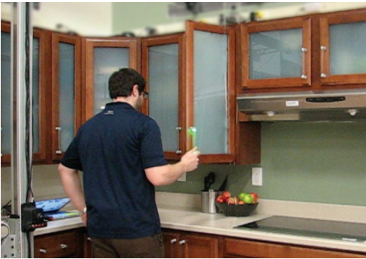
[MIDDLE] FIGURE 3-4. The Cueing Kitchen is able to prompt individuals through multistep tasks in a timely and systematic manner. PHOTOGRAPH: COURTESY OF THE HUMAN ENGINEERING RESEARCH LABORATORIES, UNIVERSITY OF PITTSBURGH.
