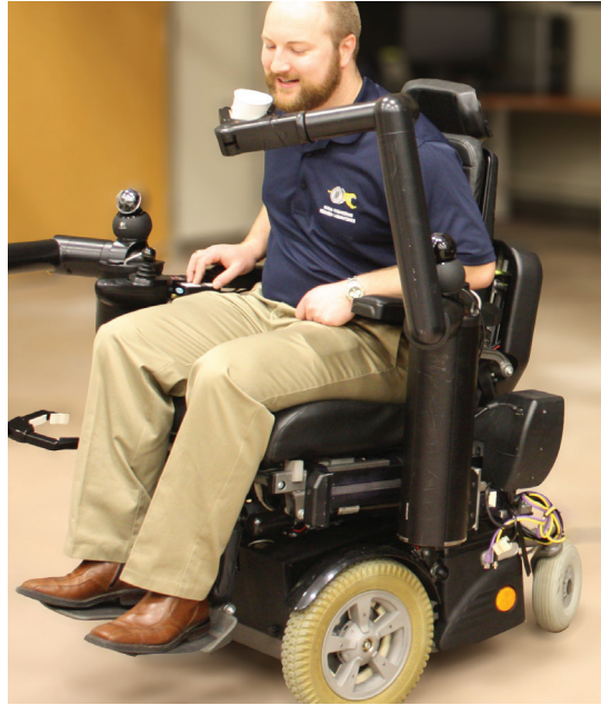
FIGURE 3-10. PerMMA is a fully robotic mobility and manipulation device for people with disabilities. It is designed to accommodate a wide variety of custom and off-the-shelf interfaces. PHOTOGRAPH: COURTESY OF THE HUMAN ENGINEERING RESEARCH LABORATORIES, UNIVERSITY OF PITTSBURGH.
