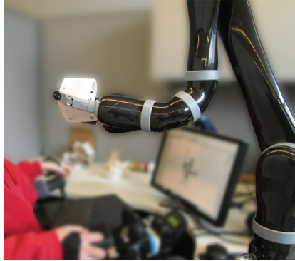
FIGURE 3-9. The KitchenBot is an overhead, track-mounted manipulator designed to aid individuals with physical impairments complete common kitchen tasks (eg, meal preparation, cleanup, etc). PHOTOGRAPH: COURTESY OF THE HUMAN ENGINEERING RESEARCH LABORATORIES, UNIVERSITY OF PITTSBURGH.
