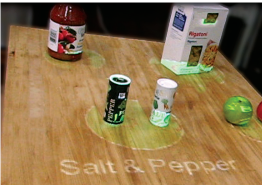
[BOTTOM] FIGURE 3-5. Interactive Island set up: Touch Interactor (area where pasta box is positioned), Count Interactor (area where salt and pepper are positioned), and Coverage Interactor (area where apples are positioned). PHOTOGRAPH: COURTESY OF THE HUMAN ENGINEERING RESEARCH LABORATORIES, UNIVERSITY OF PITTSBURGH.
