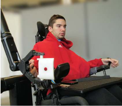
FIGURE 3-7. iARM is a commercialized wheelchair-mounted robotic manipulator with a two-fingered grip. It can be controlled by keypad, joystick, or single-button switches. PHOTOGRAPH: COURTESY OF THE HUMAN ENGINEERING RESEARCH LABORATORIES, UNIVERSITY OF PITTSBURGH.
